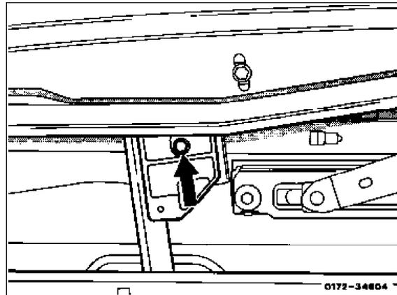
13 Adjust rear guide rail in slot in such a manner that the rear edge of the crank window abuts against sealing rubber of rear side window along entire length with door closed.
