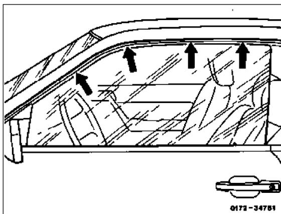
**Note:** A correction can be made by displacing rear screw on window lift guide rail and through front stop for upper lift restriction (refer to item 3).
