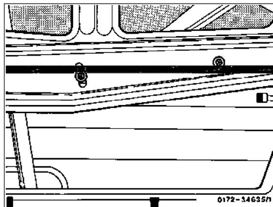
If required, the tilt and the longitudinal direction of crank window can be additionally corrected after loosening the three screws on window lifting rail.
