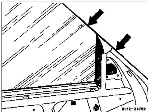
7 With window correctly adjusted, the upper edge of glass will touch the inner lip of sealing frame along entire length.
