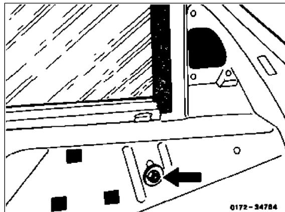
5 Loosen nut for upper angle stop, rear.
