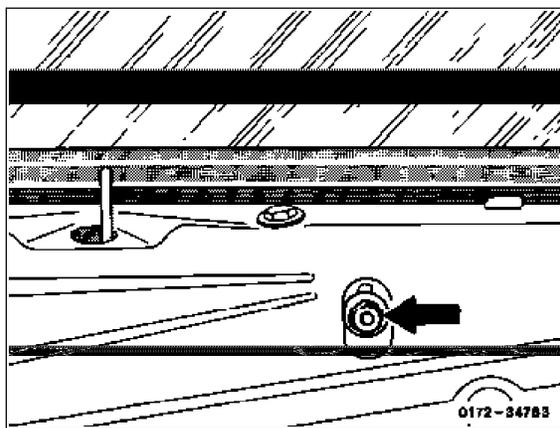
6 Close crank window until crank window is flush with front edge to guide holder.
